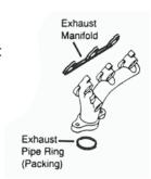
gaskets for flange-to-flange connections.
